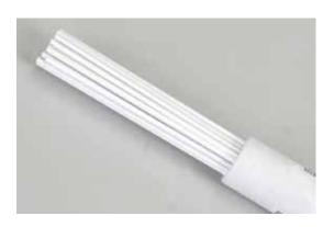
Flux coated, low furning brazing rod. Provides all properties for best tensile strength and ductility. Rod fuses well with cast iron, malleable iron, galvanized iron, steel, brass and copper. 65,000 PSI tensile strength.
